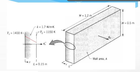
$$q_x'' = k \frac{\Delta T}{L} = 1.7 \text{ W/m} \cdot \text{K} \times \frac{250 \text{ K}}{0.15 \text{ m}} = 2833 \text{ W/m}^2$$
