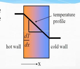
Then the rate of heat flow by conduction is:
