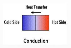
The most efficient method is conduction, which is the transfer of heat between two objects in contact. The transfer occurs as the fast-moving molecules of the hot object bump into the slower moving molecules of the cold object. The fast molecules give up some of their energy, slowing down, and this energy goes into speeding up (and thus heating up) the slow molecules.
