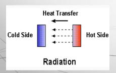
The least efficient method of heat transfer is radiation. In this case, heat moves through space without the assistance of a physical substance. This is how the Sun's heat reaches the Earth. The radiative heat is transferred directly into a solid object, but it passes readily through transparent materials such as air and glass
