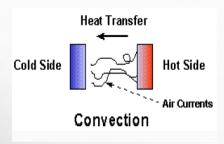
A slower method of heat transfer is convection, which occurs in fluids or gases. A cool fluid in contact with a warm solid will heat up through conduction. The warmer fluid drifts into the cooler fluid, setting up a convective current. Because material must actually be moved, convection is less efficient than conduction.
