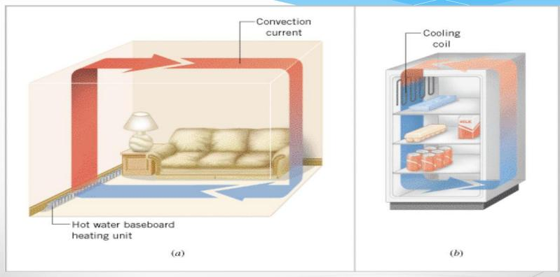
When a liquid is **heated** it becomes less dense (lighter) so it **rises**, **cold liquid** takes its place.
