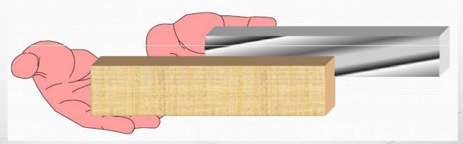
Those materials that conduct heat well are called **thermal conductors**, while those that conduct heat poorly are known as **thermal insulators**.
